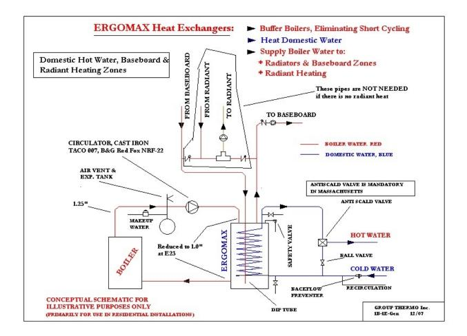
Please note that the dip tube is now built into the E23 models and the double threaded bushing is no longer needed for that model.
